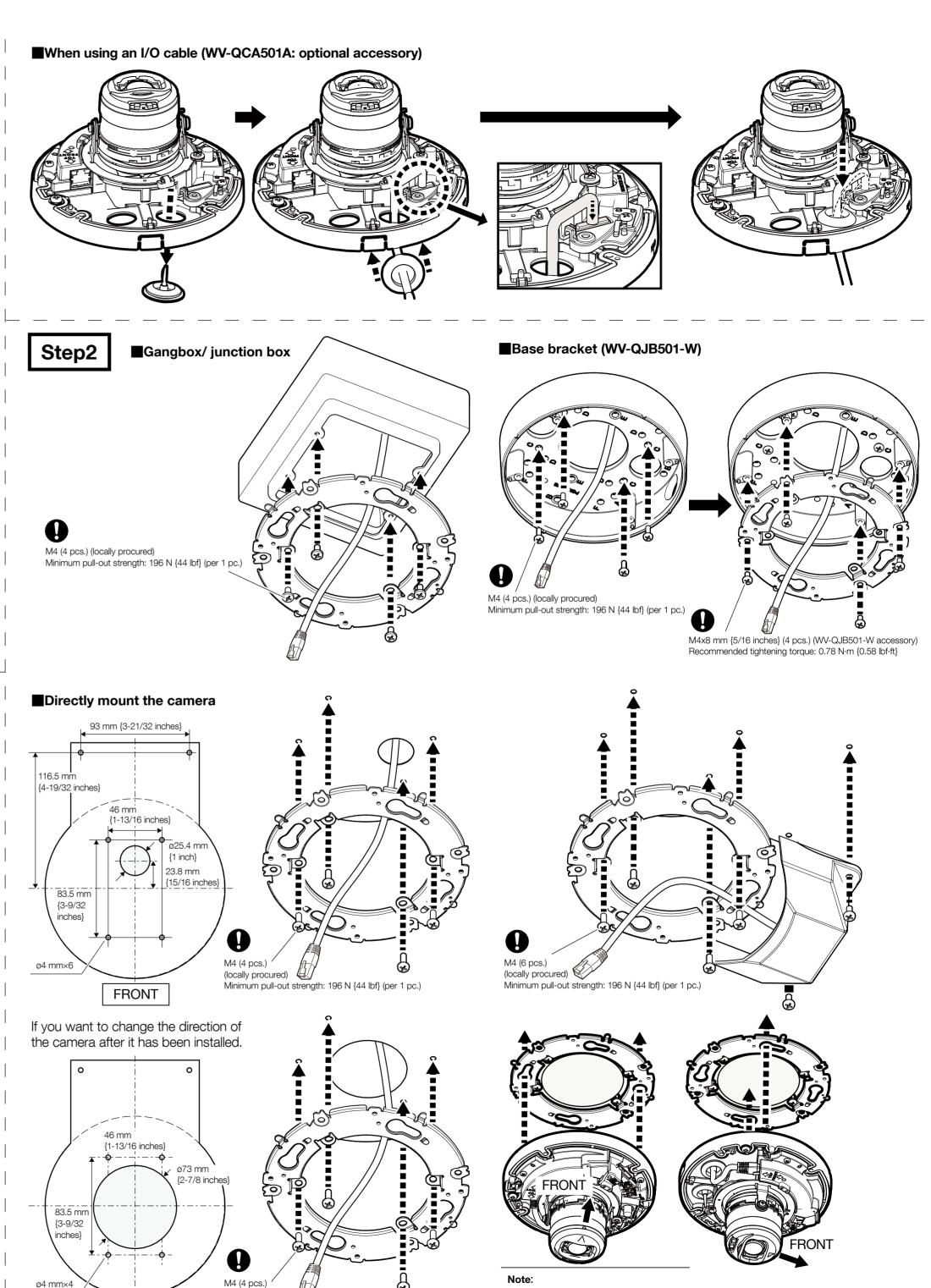
Camera can be installed in each direction.
